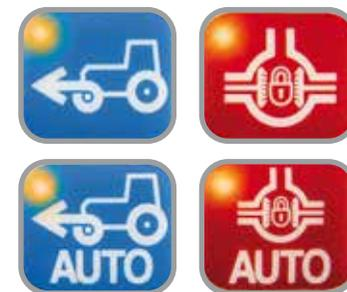
Easy-to-use buttons for all-wheel-drive and differential lock on the ICP control pad.
