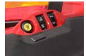
External controls are provided at the front and rear of the tractor for the hydraulic lift, PTO and an additional control unit.
