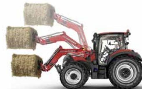
LRZ front loader with mechanical parallel guidance
